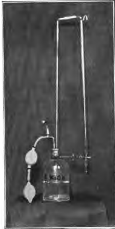
Fig. 44.—Buret for titrating media. (From Hiss and Zinsser, "Text-Book of Bacteriology," D. Appleton & Co., Publishers.)
